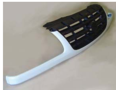
Specialty ABS plastics sold as technopolymers are increasingly being used in automotive parts.
