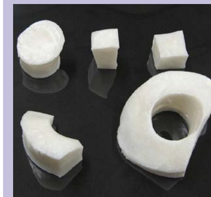
CALGRIP™ in solid state (left) and in gel state (right).
